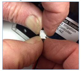
• To remove the battery, grasp the battery connector plug and socket and pull out the battery plug.
